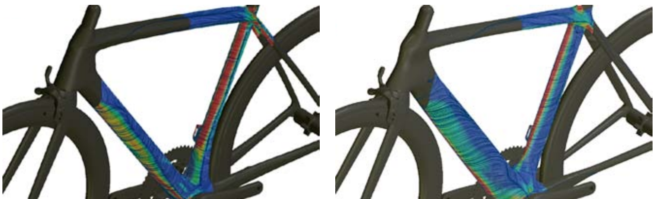
Figure 4. Proto A (left) vs. Proto X (right) — wall shear vector
