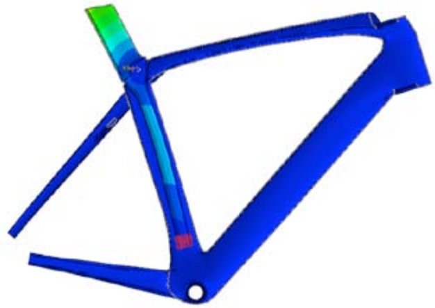
Figure 14. Vertical compliance finite element analysis of Madone prototype
