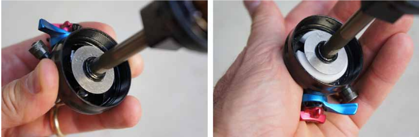
Fox offers a range of air volume spacers to change, and they're incredibly easy to install. The spacer is the white clip shown at right.
